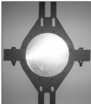
(a) Component fixture with target plate
