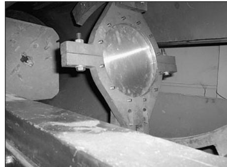
(b) Fixture with plate inside the test chamber
